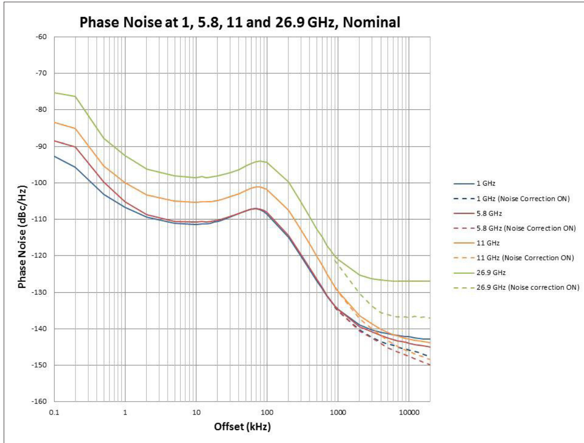
Figure 8. Nominal phase noise 1 to 26.9 GHz. Expected input level = 0 dBm, Mixer level offset = 0 dB, Pre-amp = OFF, Noise correction ON results use a counted average of 100, PeakToAverage = 5.
